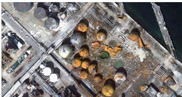
Figure 2.4. LPG tank farm in the Cosmo oil refinery was destroyed after the 2011 Tōhoku earthquake (USGS 2011)
