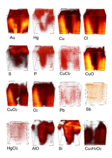
Figure 4.5. ToF-SIMS 3D imaging of the main elements and compounds revealed in the artefact.
