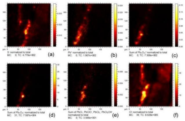
**Figure 3.20**. ToF-SIMS imaging of C6 pictorial layers. Negative maps of sulphur (a) and (f) identify the presence of vermilion (HgS) and its degradation product calomelan (Hg<sub>2</sub>Cl<sub>2</sub>) in the third layer, respectively. Positive ion maps of lead (b) and lead oxides (c), along with negative ion maps of lead oxides (d) and lead chlorides (e) identify the lead white layer in the fourth layer.
