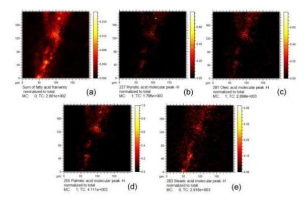
Figure 3.22. Negative ion images of fatty acids detected in the C6 cross-section. In figure 5a are summed the deprotonated molecular ion of myristic (b), oleic (c), palmitic (d), and stearic acid (e).
