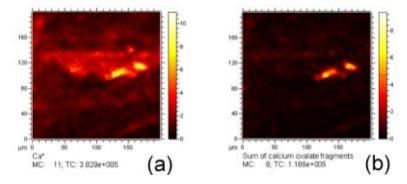
Figure 3.17. Positive ion maps of calcium (a) and calcium oxalate detected in the same area (b).
