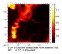
Figure 3.23. Positive ion mapping of PDMS fragments detected in C6 cross section.
