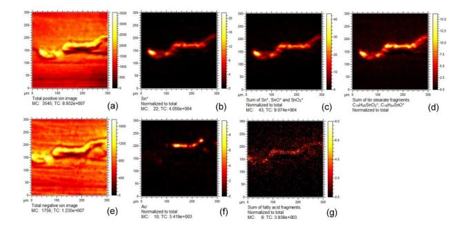
**Figure 3.6.** Imaging panel of cross section 3L. In the positive ion imaging (a), were detected the presence of tin (b), tin oxides, cassiterite and romarchite (c) and in the same area the fragmentation pattern of tin stearate (d). The negative ion images (e) shows the presence of gold leaf (f) and the fatty acid fragments distribution in the area below it, in correspondence of tin foil (g).
