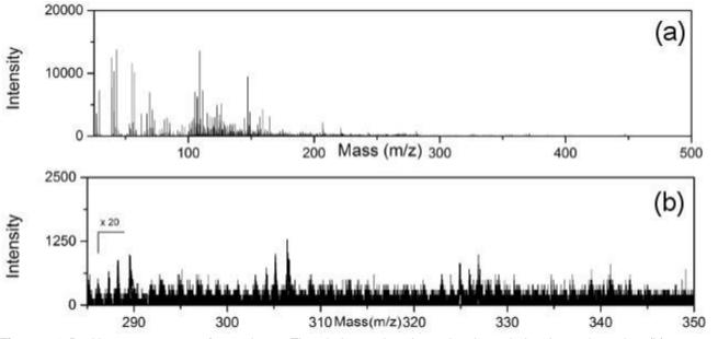
Figure 2.4. Positive mass spectra of sample 2.1. The window region shows the cluster belonging to tin azelate (b).
