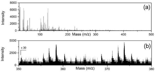
Figure 2.6. Positive mass spectra of sample 2.2. The window region shows the cluster belonging to tin palmitate (b).
