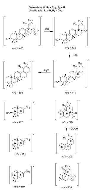
Figure 2.12. Fragmentation pathway of ursolic acid and oleanolic acid leading to the characteristic fragment ions during time-of-flight secondary ionmass spectrometry experiments
