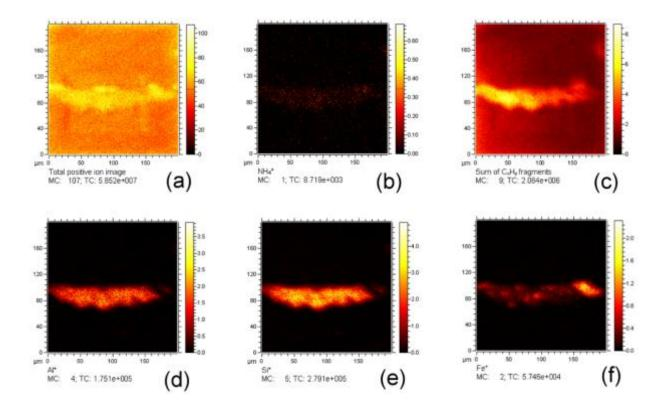
**Figure 3.15.** Main positive ion images detected in the cross section. Total positive ion image (a). The detection of  $NH_4^+$  (b) and the sum of  $C_nH_{2n-1}^+$  fragments (c) identify the presence of a proteinaceous compound in the preparation layer. Aluminium (d) silicon (e) and iron (f) identify the ochre.
