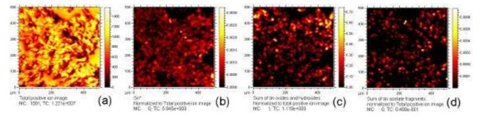
**Figure 2.5.** ToF-SIMS positive ion maps of sample 2.1. Total positive ion (a), Sn<sup>+</sup> signal (b), tin oxides cluster (c) and tin azelate (d) were normalized to the total ion image and filtered to avoid topographical effects.
