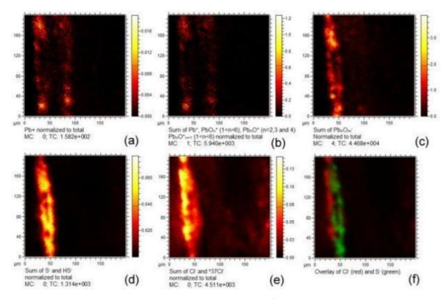
**Figure 3.25**. ToF-SIMS imaging of C7 painting layers. Ion image of  $Pb^+$  (a), positive (b) and negative (c) lead oxides belonging to lead white layer. Sulphur (d) and chloride (e) negative ion maps localize cinnabar and calomelan alteration product. The overlay of these elements is shown in Fig. f.
