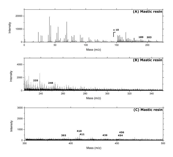
Figure A4. Positive ToF-SIMS spectrum of mastic resin: m/z 1 - 225 (A), m/z 225 – 350 (B) and m/z 350 - 500 (C).
