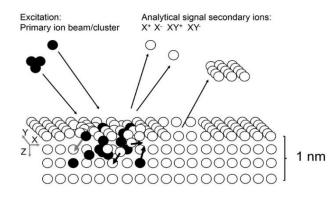
**Figure 1.1**. A schematic drawing of the secondary ion emission process initiated by the impact of a primary ion. Extensive fragmentation occurs near the collision site producing mainly atomic particles. Away from the point of impact collisions become less energetic resulting in the emission of larger molecular fragments
