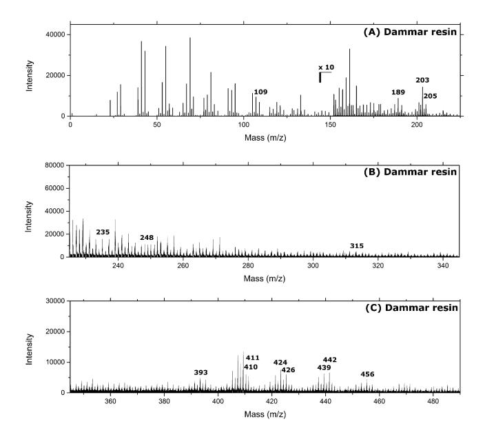
**Figure A3.** Positive ToF-SIMS spectrum of dammar resin:  $m/z \ 1 - 225$  (A),  $m/z \ 225 - 350$  (B) and  $m/z \ 350 - 500$  (C).
