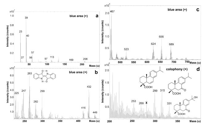
Figure 3.10. ToF-SIMS spectra in positive mode of sample 1 (a,b,c) and fresh colophony reference sample (d).
