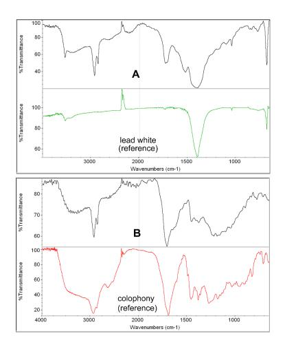
**Figure 3.1.** Micro-FTIR spectra of sample 2 compared to reference spectra. (A) White portion: reference lead white and (B) gold varnish portion: reference colophony
