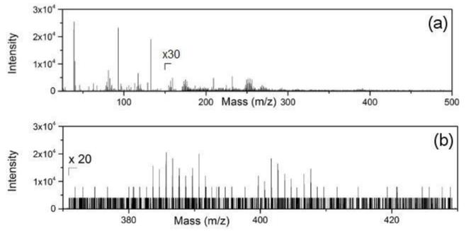
Figure 2.8. Positive mass spectra of sample 1.3. The window region shows the cluster belonging to tin stearate (b).
