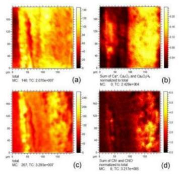
**Figure 3.24**. ToF-SIMS imaging of C7 cross-section. Positive and negative ion maps of the area analyzed (a-c). Calcium oxides (b) and cyanate group (d) characterize the preparatory layer.
