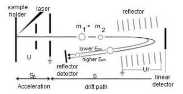
**Figure 1.3.** Schematic representation of time of flight (ToF) analyzer. The accelerated molecular ions leave the sample holder with the same kinetic energy and travel along the linear flight tube with different velocities according to their m/z. In a reflectron TOF analyzer the ion separation resolution is improved. The spread of flight times of the ions with the same m/z, caused by spread in kinetic energy of these ions, is diminished.
