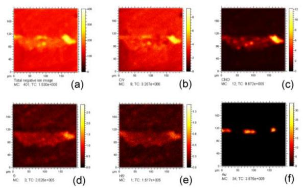
**Figure 3.16.** Main negative ion images detected in the cross-section. Total negative ion image (a). Maps of  $CN^{-}$  (b),  $CNO^{-}$  (c),  $S^{-}$  (d) and  $HS^{-}$  (e) could indicate the presence of a proteinaceous compound in the ochreys layer as binding media. The gold leaf was detected on the top of the sample (f).
