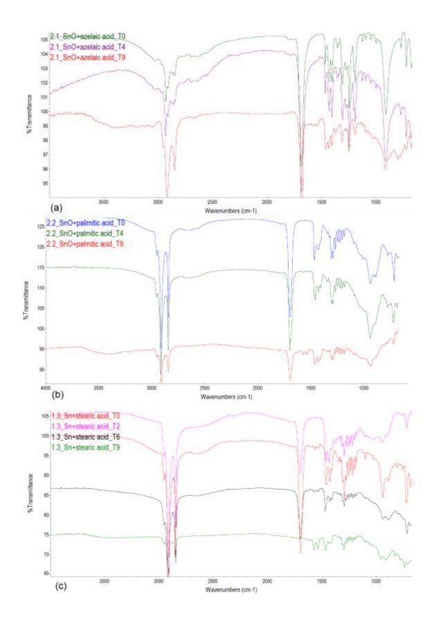
Figure 2.2. FTIR spectra of tin azelate sample 2.1 (a), tin palmitate sample 2.2 (b), and tin stearate sample 1.3 (c).
