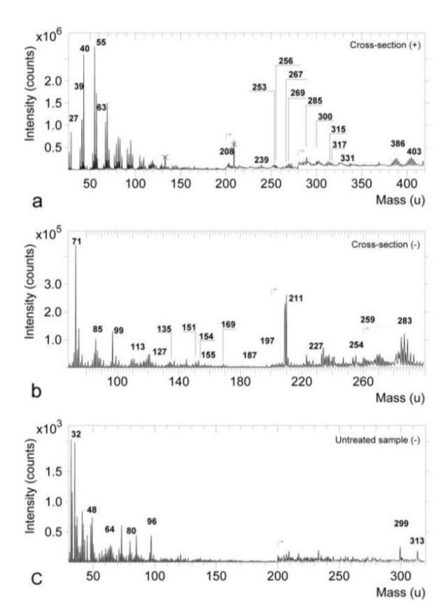
**Figure 3.2.** Relevant time of flight secondary ion mass spectrometry spectra of fresco cross section: (a) positive ion mode, (b) negative ion mode, and (c) negative ion mode of red lake area (untreated sample).
