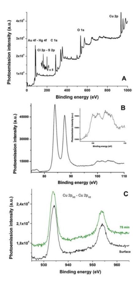
**Figure 4.3.** XPS wide scan of the surface of the gilded clasp with identification of the main peaks of C, O, Cl, S, Cu, Au and Hg; Au 4f  $_{7/2}$ -Au 4f  $_{5/2}$  and Hg 4f  $_{7/2}$ -Hg 4f  $_{5/2}$  core level spectra; Cu 2p  $_{3/2}$ -Cu 2p  $_{1/2}$  core level spectra, A, B and C, respectively.
