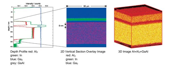
**Figure 1.5**. Example of reconstruction possibilities from raw data. The sample is a GaAs/AlGaAs superlattice. A volume of 60 x 60  $\mu$ m<sup>2</sup> (surface area) x 400 nm (depth) was analysed. The 2D section and the 3D image are reconstructed from depths of 130 nm to 340 nm (<u>www.iontof.com</u>).
