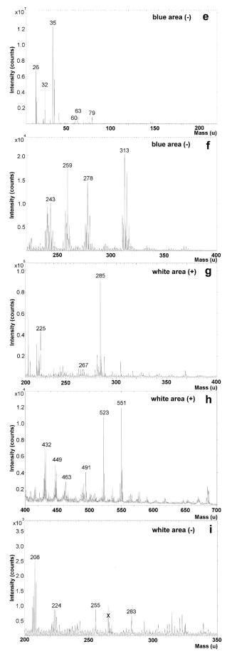
Figure 3.11. Negative secondary ion spectra of sample 1 (e,f) and sample 2 (i). ToF-SIMS spectra in positive mode of sample 2 (g,h).
