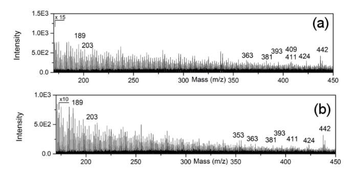
**Figure 2.16.** ToF-SIMS Positive mass spectra (range m/z 170-450) of reference pitch derived from bark of a *Betula* spp. (a) and archaeological blackish sample collected from the sickle (b).
