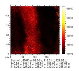
Figure 3.26. ToF-SIMS negative imaging sum of fatty acids deprotonated molecular ions, detected in C7 cross-section.
