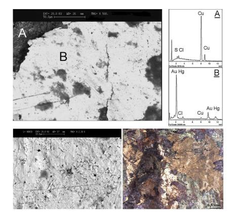
**Figure 4.1**. BSE images and EDS spectra of a gilded clasp for bridles. The results reveal that the plating is composed of small rounded and flattened grains of gold with a low amount of mercury. The diameter of the grains range from 1  $\mu$ m to 3  $\mu$ m. OM micro-graph shows the presence of erupting cuprite (Cu<sub>2</sub>O) that has caused the partial removal of the plating.
