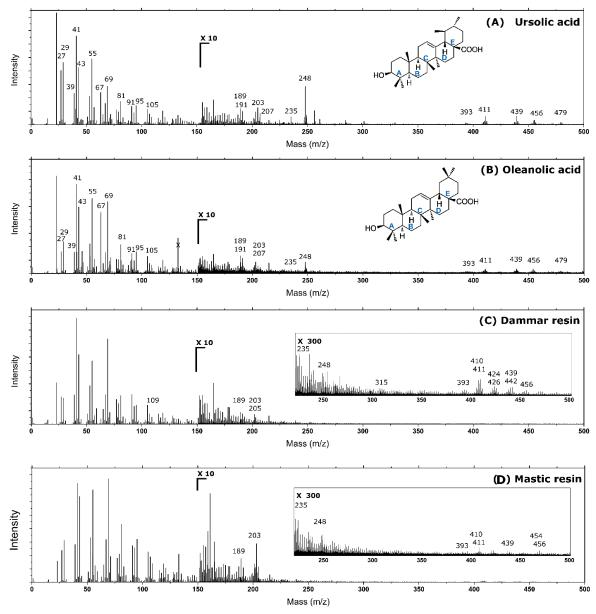
**Figure 2.11.** Positive time-of-flight secondary ionmass spectrometry spectra (m/z 1-500) of ursolic acid (A) oleanolic acid (B) dammar (C) andmastic resins (D).
