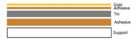
**Figure 2.1**. Schematic representation of the so called *composite lamina* technique. The tin foil is pasted to a support with an adhesive mixture and superimposed by a gold leaf, which is also pasted with the same oil-resinous compound.
