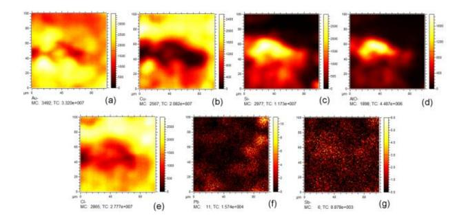
Figure 4.6. ToF-SIMS negative ion images of the sample surface.
