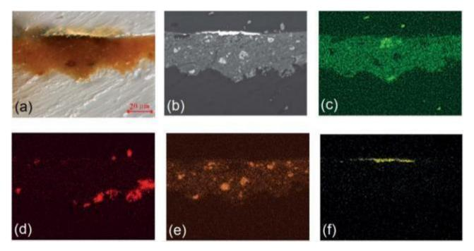
Figure 3.14. SEM mapping of main elements found in cross-section. Visible light optical image (a) and back scattered electron image of cross-section (b). X ray maps of silicon (c), calcium (d), iron (e) and gold (f).
