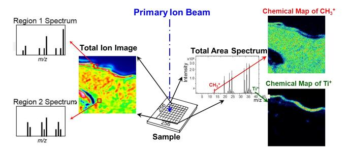
Figure 1.4. Principles and schematic representation of Time-of-Flight Secondary Ion Mass Spectrometry.
