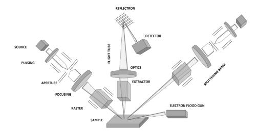
**Figure 1.2**. Schematic drawing of a SIMS instrument with a TOF analyzer. The primary ion source, sample, and flight tube are kept under UHV. The mass of the detected ions is determined by the flight time of the ion between the extractor and the detector. The reflectron helps compensate for energy and angular dispersion that can occur during the emission process.
