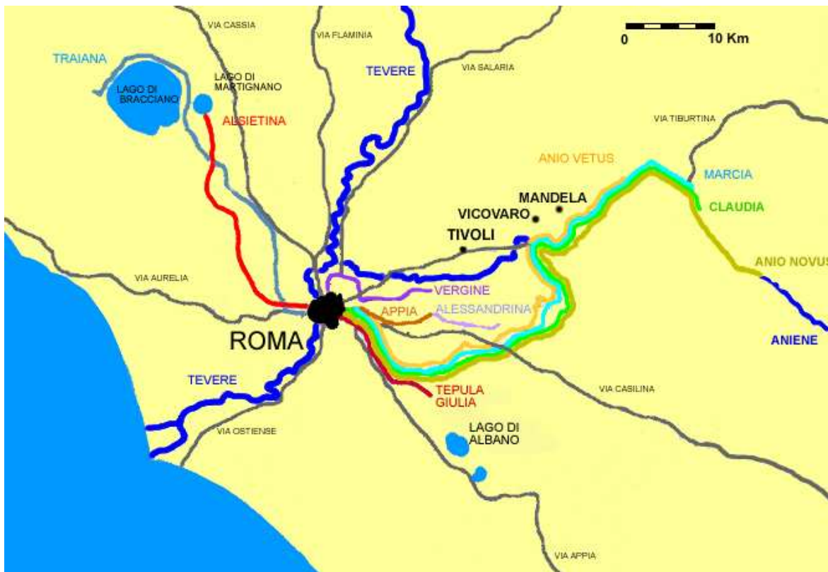
Fig. 2.55: The network of eight aqueducts built in ancient Rome is show; at the end of II century, they used to bring to the City around 10 m 3 /s.
