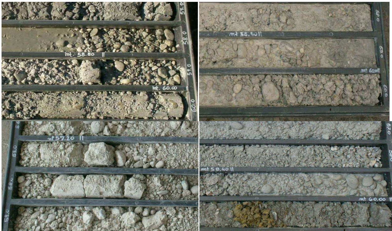
Fig 2.33: Pictures of cores drilled in three different sites along the path of “C” subway line (“Metro C”)
