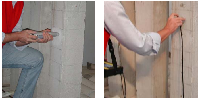
Figure 3.1: sclerometric test (left) and ultrasonic test (right) on a column of the portal
