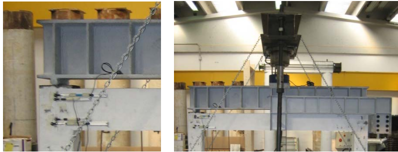
Figure 7.4: structure designed to apply the gravity load on columns
