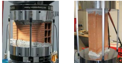
Figure 2.14: hollow brick compression tests, compression orthogonal to holes (left); compression parallel to holes (right)
