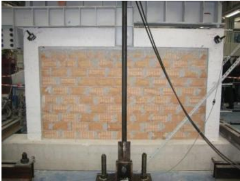
Figure 7.12: instrumentation of the infilled portal, side 2
