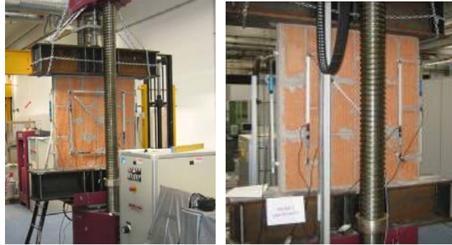
Figure 2.45: equipment for compression test parallel to holes on hollow brick walls (front and back view of the panel)
