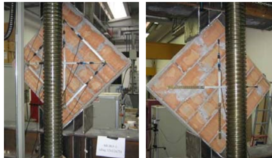
Figure 2.50: equipment for diagonal compression test half-full brick walls (front and back view of the panel)
