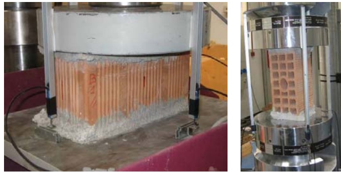
Figure 2.20: half-full bricks compression tests, compression parallel to holes (left); compression orthogonal to holes (right)
