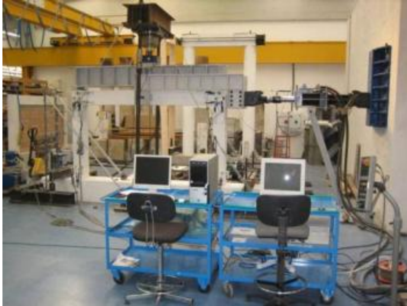
Figure 7.8: set-up of the experimental test on the bare portal
