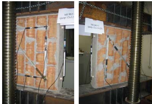
Figure 2.49: equipment for compression test orthogonal to holes on half-full brick walls (front and back view of the panel)
