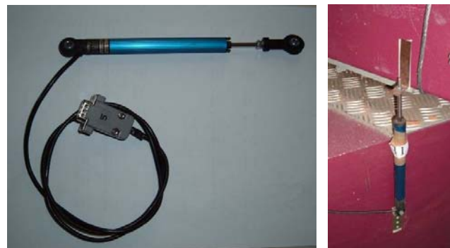
Figure 2.35: transducer adopted to measure deformations (left), the external transducer installed (right)
