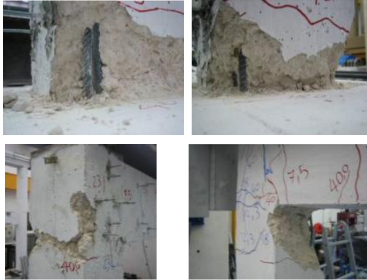
Figure 7.15: portal F_{n1} , damage to the top of the columns (collapse)
