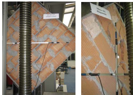
Figure 2.96: diagonal compression test, front and side view of collapse
