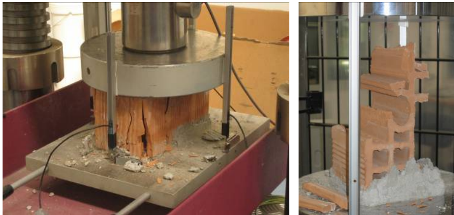
Figure 2.21: failure of a sample of half-full bricks, compression parallel to holes (right) and orthogonal holes (left)
