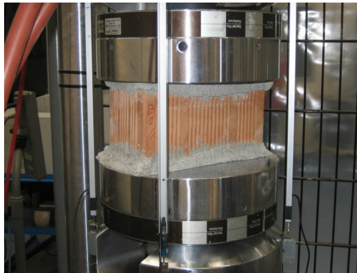
Figure 2.6: characteristics of the system for compression tests on bricks
