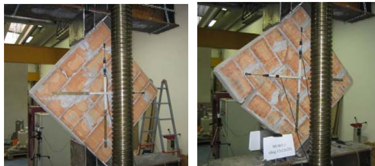
Figure 2.67: diagonal compression test, initial phase and collapse
