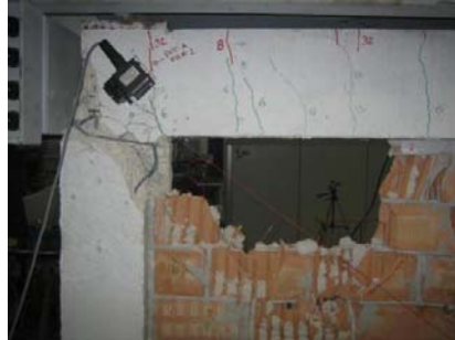
Figure 7.28: portal frame F_{t1} , detail of the structure following collapse
