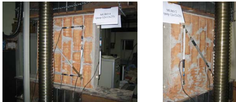
Figure 2.66: compression test orthogonal to holes, initial phase and collapse
