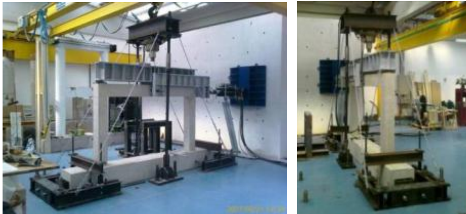
Figure 7.2: the test system set-up on the portal F_{nl}
