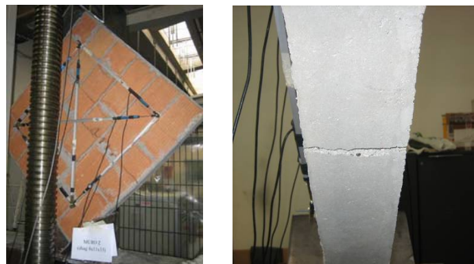
Figure 2.56: diagonal compression test, front and side collapse view
