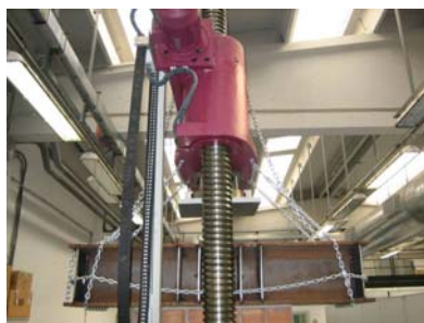
Figure 2.34: suspension system of the upper steel profile
