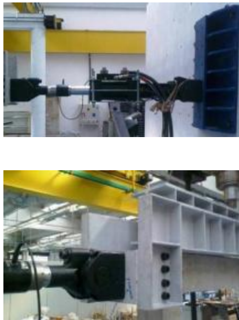
Figure 7.3: details of the jack M_h installed on the contrast wall (top) and on the portal (bottom)
