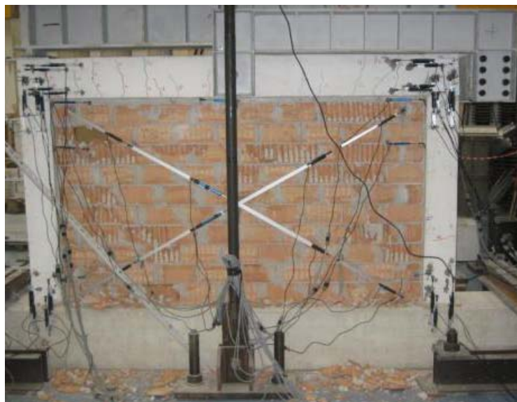
Figure 7.27: portal F_{11} , infill damages during the experimental test (after having achieved maximum load)
