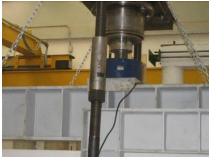
Figure 7.13: loading cell inserted under the hydraulic jack
