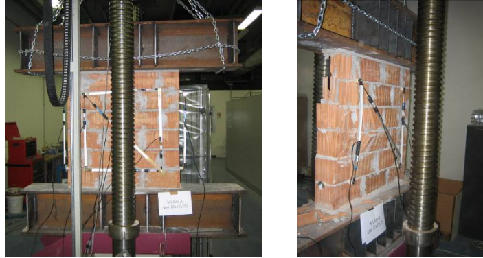
Figure 2.65: compression test parallel to holes, initial phase and collapse
