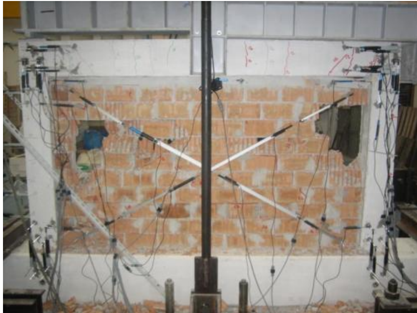
Figure 7.30: portal frame F_{11} , infill damages during the experimental test (after having achieved maximum load)
