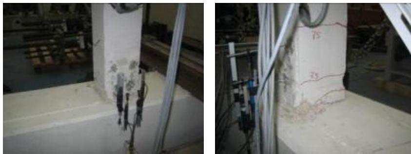
Figure 7.14: portal F_{n1} , damage to the base of the columns (top displacement of 30\text{ mm} )
