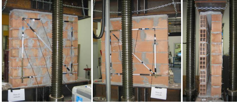
Figure 2.51: equipment for vertical compression on double panel walls (front and back view of the panel)
