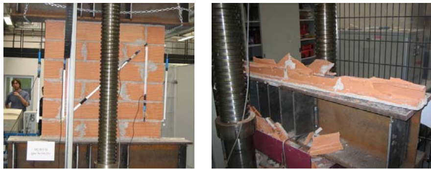
Figure 2.55: compression test orthogonal to hole, initial phase and collapse
