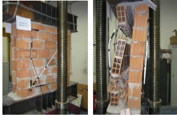
Figure 2.94: compression test parallel to holes, initial phase and collapse
