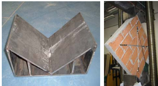
Figure 2.33: diagonal compression tests set up, steel supports for diagonal compression tests (left), wall ready to be crashed inside the press (right)
