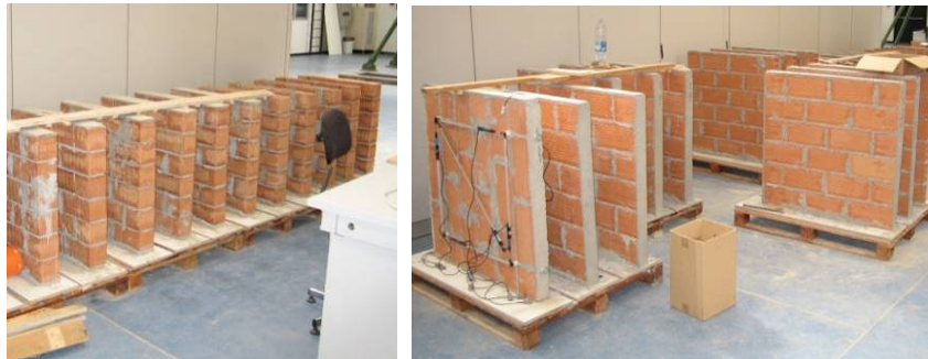
Figure 2.26: walls specimens, walls of half-full bricks (left), walls of hollow bricks (right)
