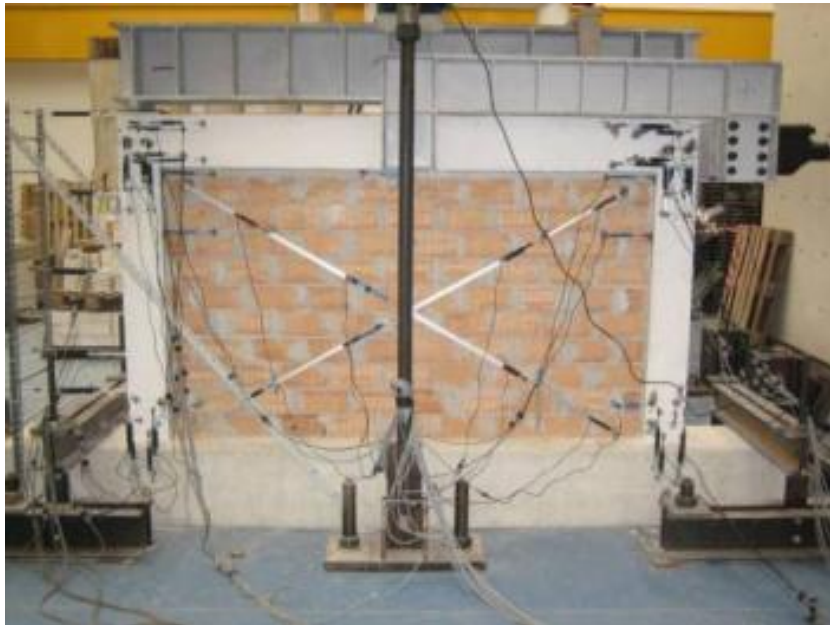
Figure 7.11: instrumentation of the infilled portal, side 1
