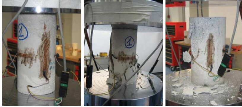
Figure 2.10: Compression tests on mortar cylinders
