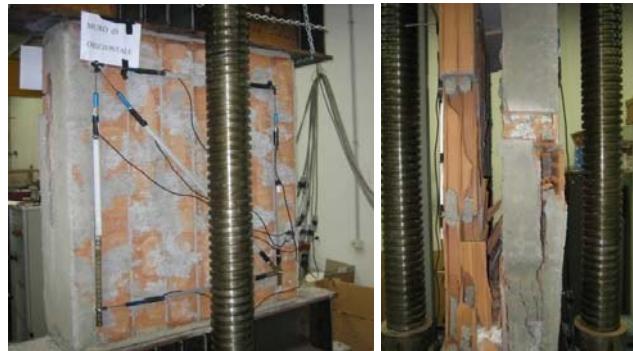
Figure 2.95: compression test orthogonal to the holes: initial phase and collapse
