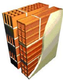
Figure 2.3: types of infill walls: a) walls with double panel with air space b) plain wall
