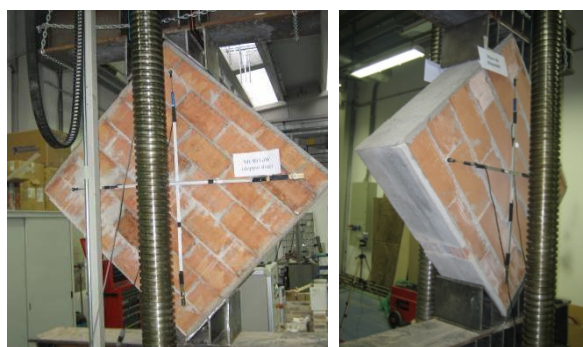
Figure 2.53 equipment for diagonal compression on double panel walls (front and back view of the panel)
