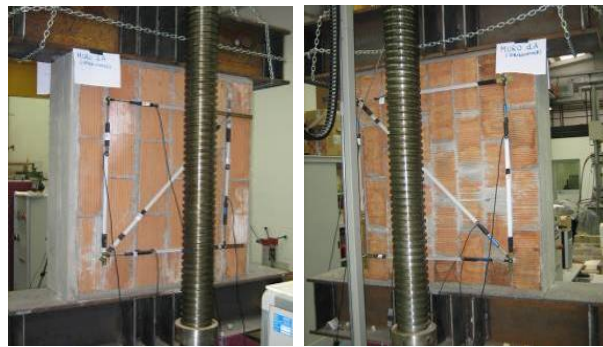
Figure 2.52: equipment for horizontal compression on double panel walls (front and back view of the panel)
