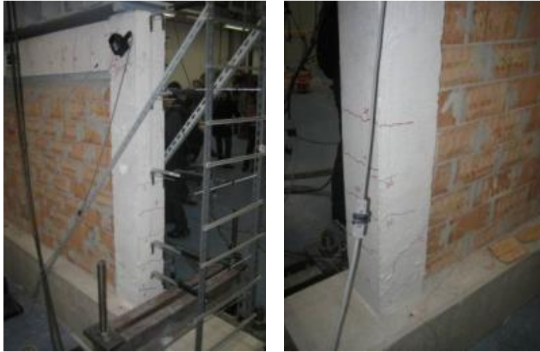
Figure 7.24: portal F_{tl} , superficial cracks along columns height
