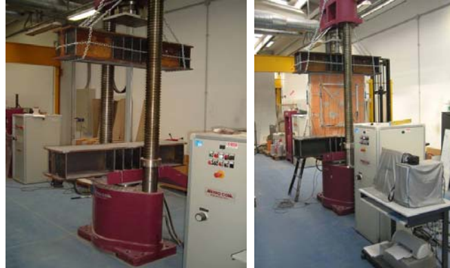
Figure 2.32: equipment set up for vertical compression tests: the steel profiles fitted onto the Metrocom 3000 kN press (left), a wall ready to be crashed inside the press (right)
